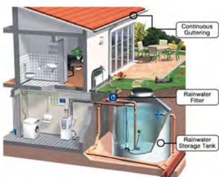
Rainwater harvesting system
